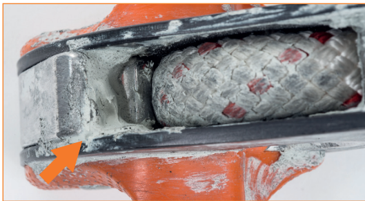
Regulator with cam jammed due to build-up of foreign matter.
