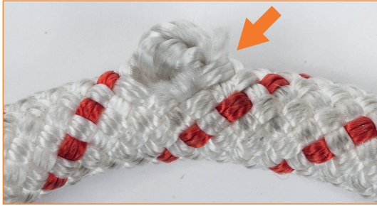
Rope core protruding.
