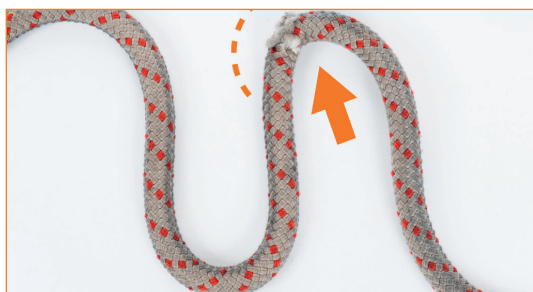
Damaged rope. Note the difference in curvature between the undamaged portion (constant curvature, below left) and the damaged portion (uneven curvature, above right).
