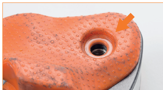
Regulator with missing screw.
