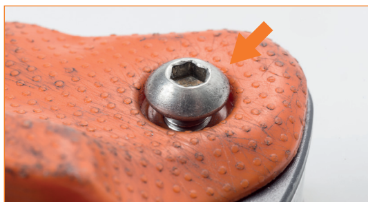
Regulator with loose screw.
